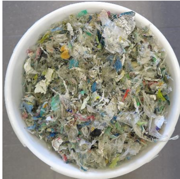
r-LDPE Film contains 10-15% water without de-watering aid
