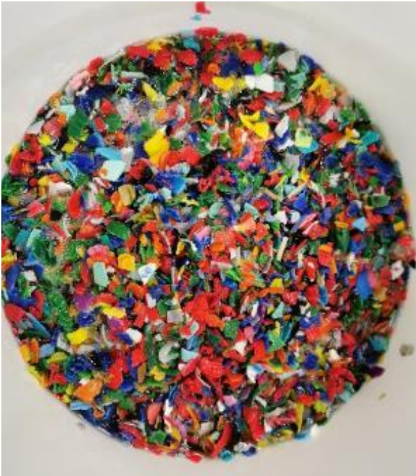
r-HDPE or r-PP Flakes contain 5-10% water without de-watering aid
