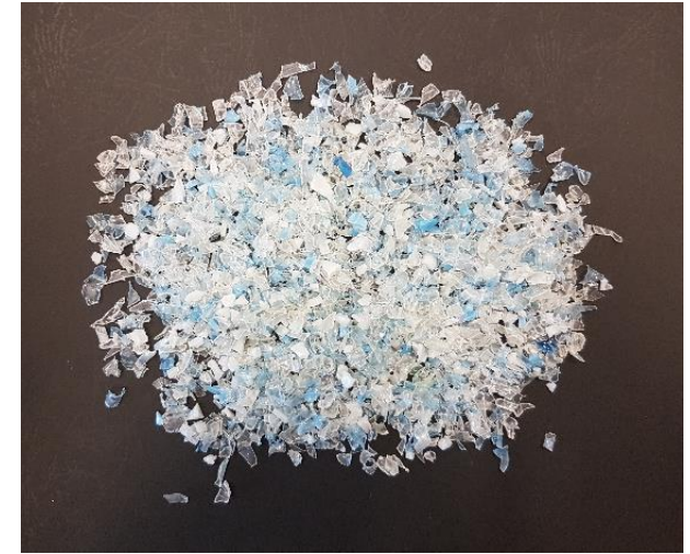
r-PET flakes contain 0.5-2.0% water without de-watering aid
